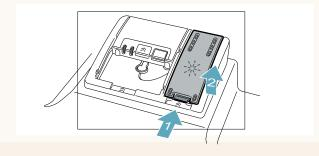
2. Add liquid rinse aid to the dispenser 1b until it is full. Do not overfill. Avoid spilling into air vent hole.
